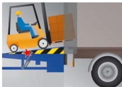
Safeguard emergency stop with two cylinders.
