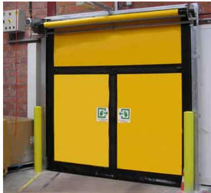
Crawford 9110 EM high speed door Designed with an integrated emergency exit for heavy-duty inside operations. Max. Size (WxH): 5500 x 5500 mm Operating speed: Opening: up to 2.0 m/s Closing: 1.0 m/s
