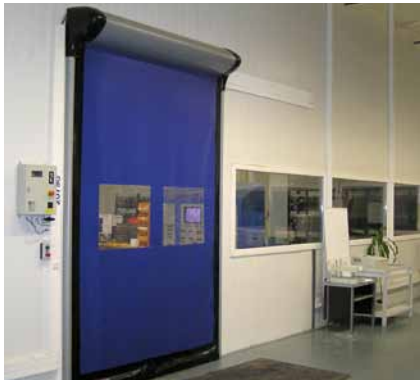
Crawford 9220 AT high speed door A compact airtight door with integrated motor suitable for inside environments such as cleanrooms. Max. Size (WxH): 3500 x 3500 mm Operating speed: Opening: up to 2.7 m/s Closing: 0.5 m/s
