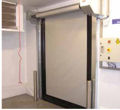
Crawford 9110 FR high speed door Designed for freezer applications, allowing efficient traffic flow while minimizing temperature variations. Max. Size (WxH): 4500 x 4500 mm Operating speed: Opening: up to 2.4 m/s Closing: 1.2 m/s
