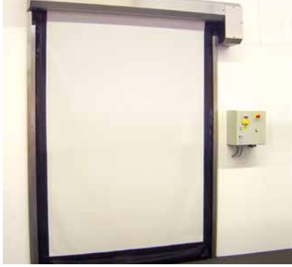
Crawford 9210 HY high speed door For special applications like the food industry where the demands on hygiene are high. The complete door frame* is made of stainless steel. Max. Size (WxH): 4000 x 4000 mm Operating speed: Opening, up to 1.2 m/s Closing, 0.5 m/s
