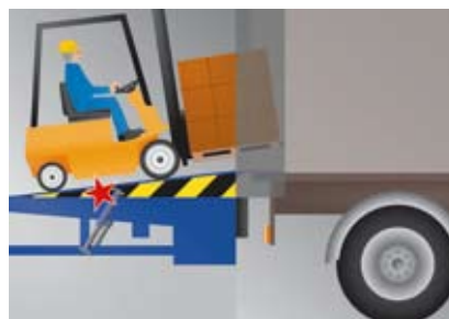
Safeguard emergency stop with two cylinders.
